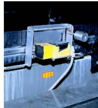
That's exactly why TURCK's analog sensors are used in many applications requiring more than simple digital positioning control.
