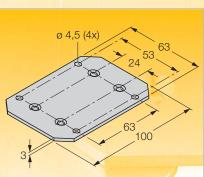
The mounting panel FTCI-MP01AL (Ident-no. 6870040) can be attached to the sensor housing (matching screws supplied). The panel is used for front mounting.
