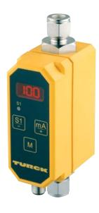
The thermal inline flow rate sensors FTCI are equipped with a 3-digit 7-segment display to indicate the actual flow rate in [l/min]. These sensors are particularly suited for flow rate monitoring within cooling circuits due to their fast response times within seconds and their reliable and stable value display, even if the application is exposed to strong temperature fluctuations.
